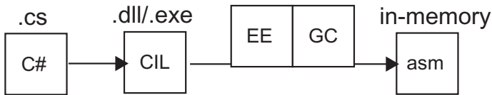
Figure 4-1. Source code (text files) are being compiled into Common Intermediate Language (binary files). Then on a target machine with .NET runtime installed, it is being run by the runtime itself. It consists of two main units: Execution Engine (EE) and Garbage Collection (GC). EE is taking CIL from the binary files and transforms it in memory to the machine code.
